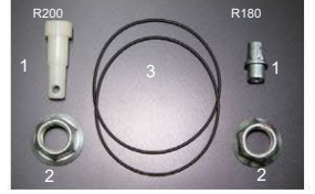
R200/R180 Differential parts R200 R180 1.Breather ¥320 ¥310 2.Pinion locknut ¥1,510 ¥360 3.Retainer O-ring SET — ¥540 (Updated 2025.10.30)
