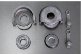
Rear Wheel Cylinder Cup Kit Part Number: 18090 (Check the boot shape) Size: 13/16 (NABCO) Compatible with: GC110, KHC130 Price: ¥980
