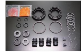
DR30 Turbo (late model) R caliper seal kit Part number: 06P26 Applicable period: 1983.2-1985.10 Price: ¥7,250 (5.4.28)
