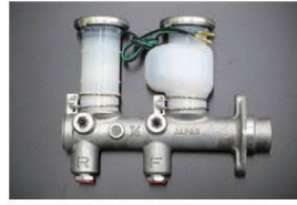
P330 Brake master cylinder size: 7/8 (Nissan genuine Nabco) Compatible with: Rear drum vehicles (L20/L28) (75.6-79.5) Price: ¥88,000 (Updated 2026.06.04)
