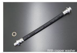
S30, S31, PS30 genuine clutch hose *Total length: 230mm (including thread) *Compatible with: S30, S31, PS30 Price: ¥3,270 (Updated 2026.04.09)
