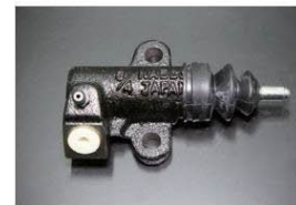
FJ20 Standard release cylinder Compatible with: All FJ20 vehicles Size: 3/4 (automatic adjustment) Price: ¥7,530 (Updated 2026.04.09)
