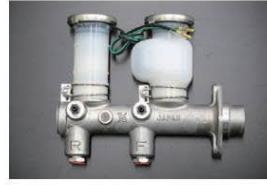
GC110 Brake master cylinder size: 7/8 (Nissan genuine Nabco) Compatible with: GC110 late model, GC111 (rear drum 75.10-77.7) Price: ¥88,000 (Updated 2026.06.04)
