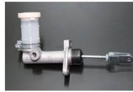
5/8 clutch master cylinder Compatible with: GC210, GC211 (for GT, GTX) Size: 5/8 Price: ¥11,000
