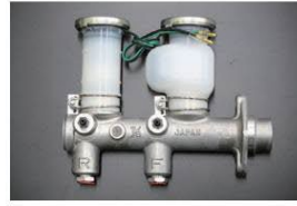
GC110 Brake mastercylinder size: 7/8 (Nissan genuine Nabco) Compatible with: GC110 late model, GC111 (rear drum 75.10-77.7) Price: ¥50,000
