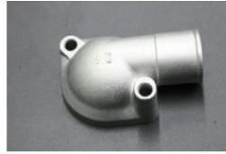
Genuine L-type thermo cover (2 bolts) Fits: L-type Vehicles: S30, GC10, etc. Price: ¥2,250
